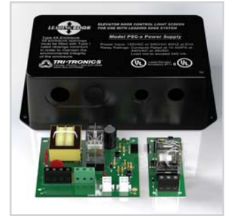
PSC-5NW Power Supply with Nudging In waterproof housing
