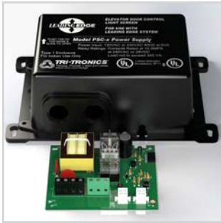
PSC-4 Power Supply In non-metallic housing
