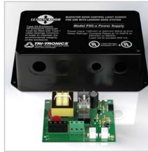
PSC-5W Power Supply In waterproof housing
